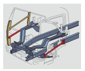
10 Fuso RISE Body with door impact beam, front box structure and reinforced cab floor main sill.
