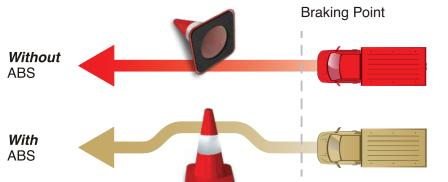
ABS help to maintain control of the vehicle during emergency braking situations, and enable proper steering around obstacles.
