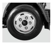
09 Tubeless tyre providing longer tread life and gentle deflation in case of puncture.
