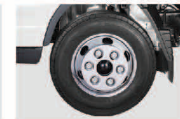
10 Tubeless tyre providing longer tread life and gentle deflation in case of puncture.
